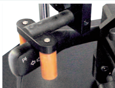
Checking operating torque of steering column controls
