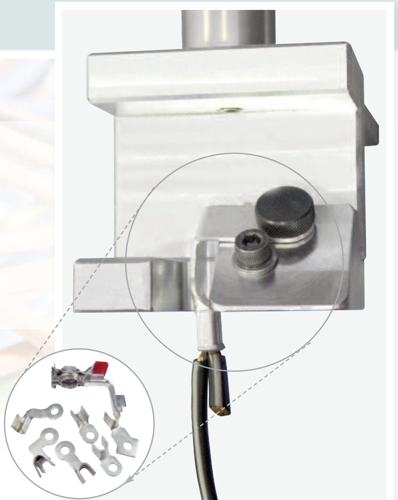
Tensile testing of crimped and welded joints
