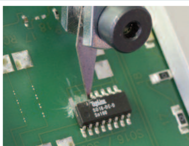
Pull-off strength of circuit board components
