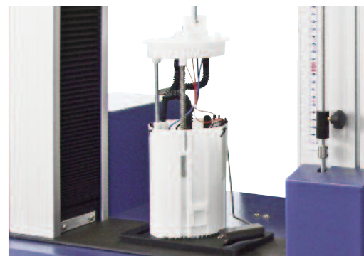
Spring testing in a fuel pump assembly
