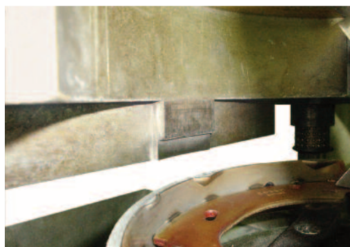
Measuring shear strength of brake linings
