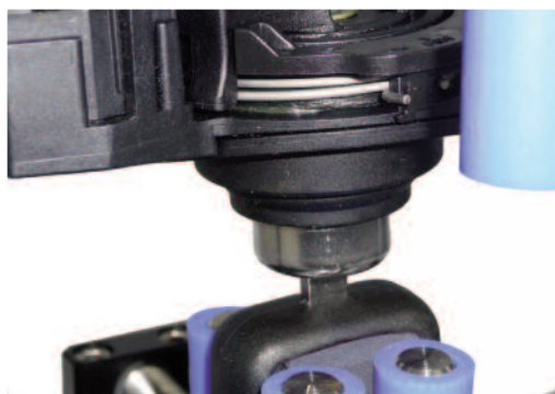
Measuring torsion-sprung lock effort
