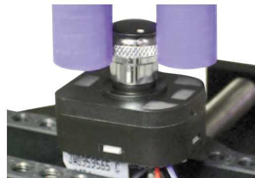
Torque testing of rotary switch
