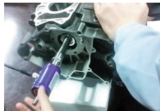
Torque testing a motor shaft
